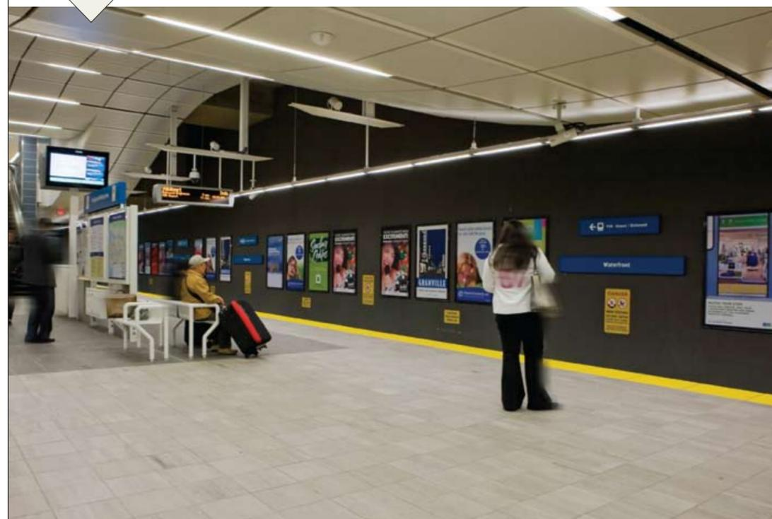
daylight harvesting, resulting in an overall lighting power density of 0.64 watts per sq. ft., 36% less than the ASHRAE 90.1-2004 energy standard’s 1 watt per sq. ft. With 20/7 operation, energy savings top 1.5 million kWh, which earned a \$120,000 utility rebate.
